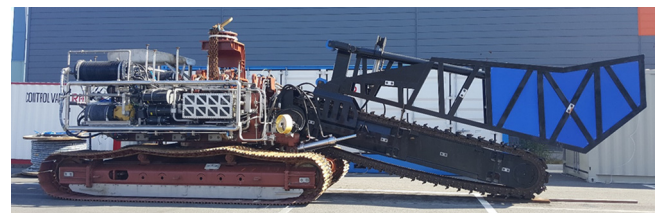
Fig. 1 Underwater construction robot URI-R
